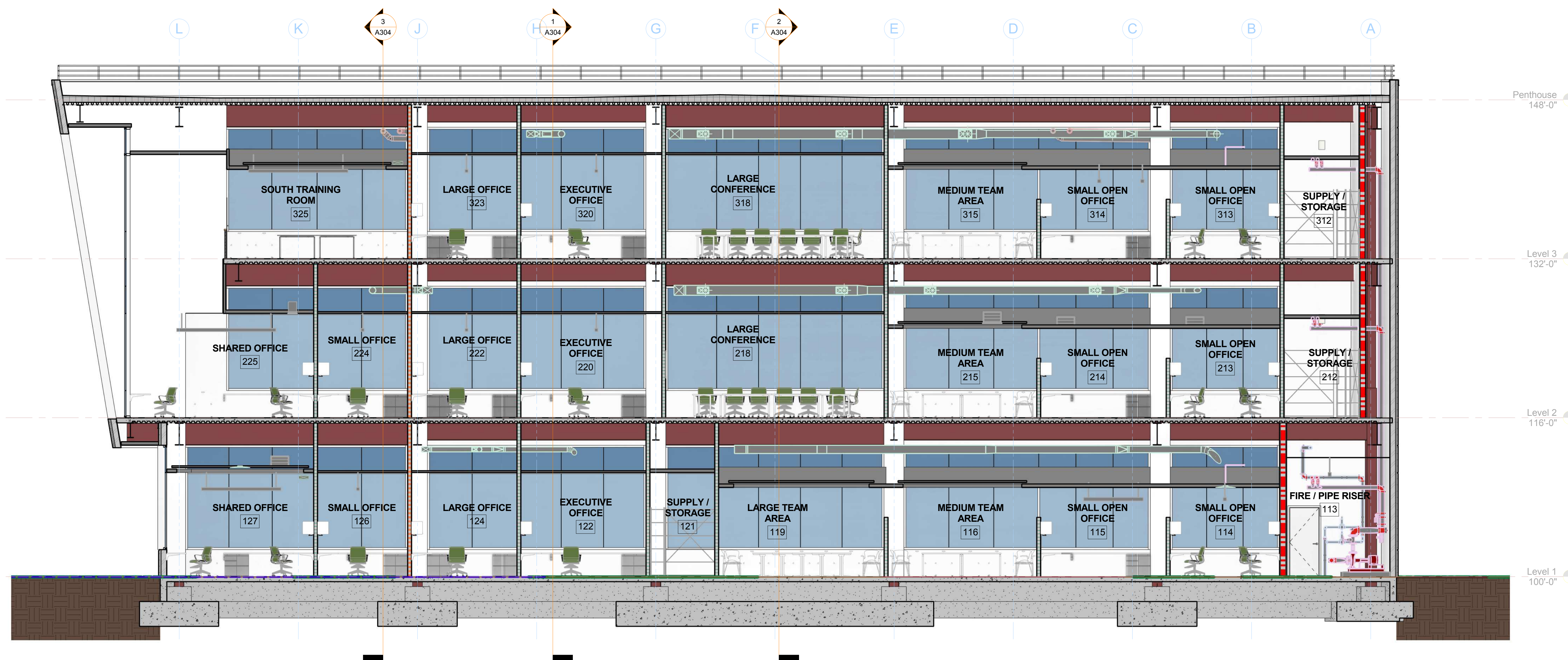
4 South Offices East-West Section SCALE= 3/16" = 1'-0"
